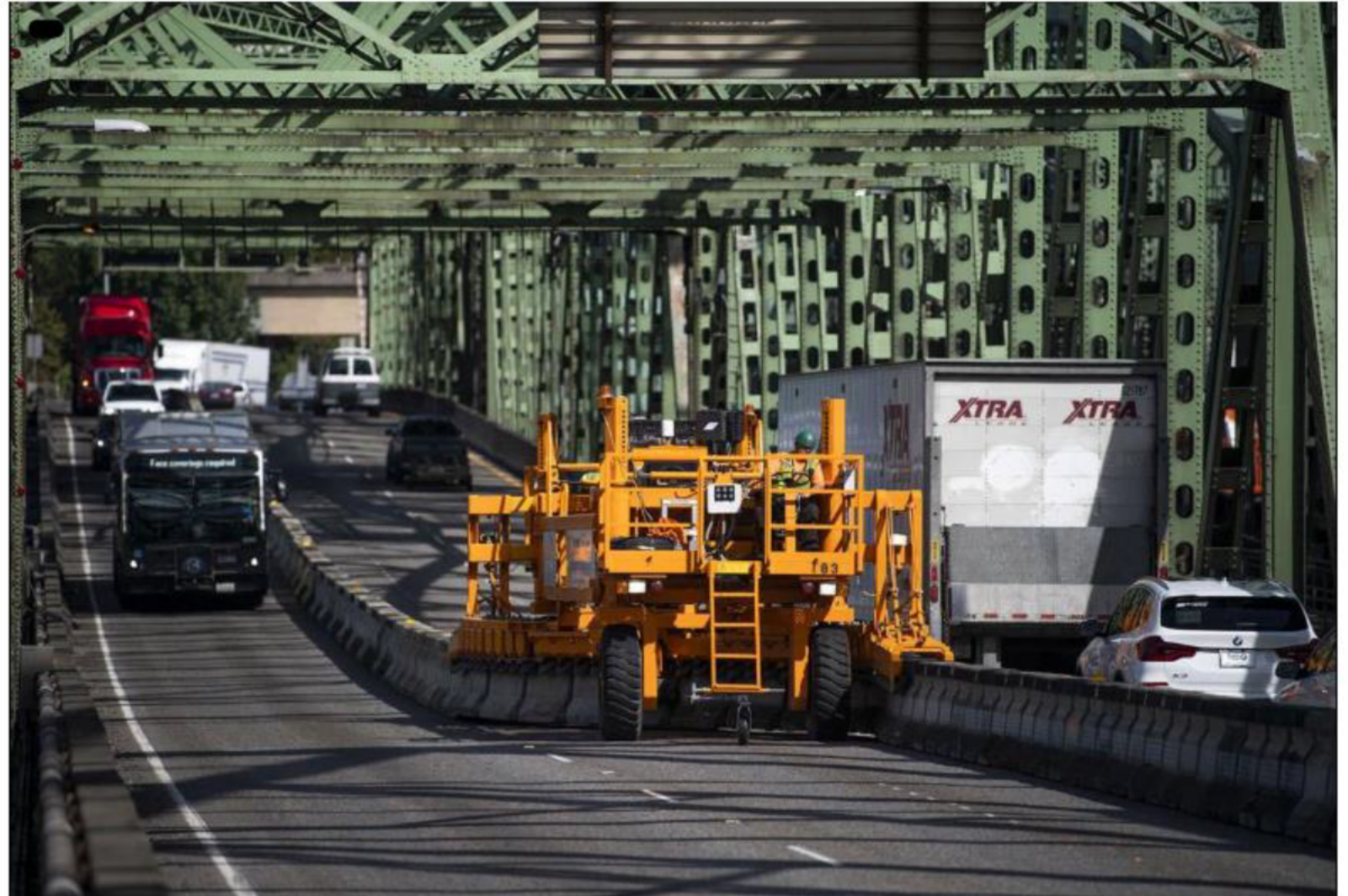
Just like a zipper, this machine switches barriers on commuter lane on the I-5 bridge between Vancouver and Portland.
